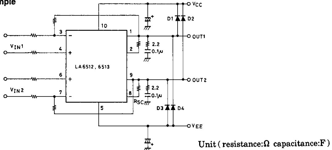
Note: When driving an inductive load, a D1 to D4 protective diode should be installed.
