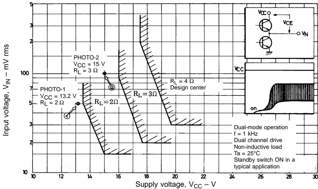
Strong signal input after switch-ON is OK.
