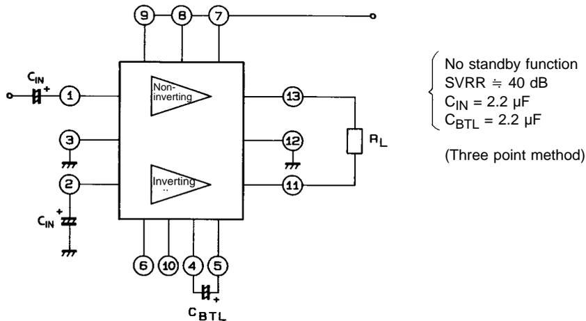
Dual-mode short-circuit test circuit
