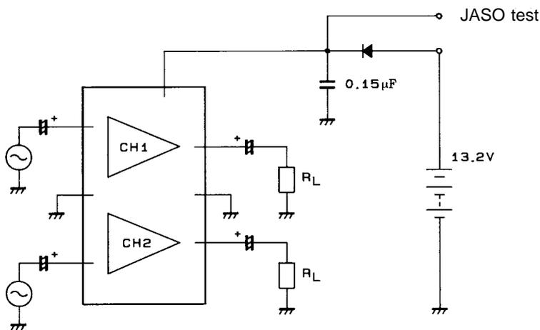
The power supply line positive surge breakdown margin has been increased by using the built-in overvoltage protection circuits ( $V_{CCX} = 28$  V) to cut off all bias circuits/change the base-emitter reverse of the output stage. In other words, the breakdown margin is being raised by changing output stage groups that operate as the  $V_{CEO}$  ( $V_{CER}$ ) type to the  $V_{CES}$  ( $V_{CBO}$ ) type.
