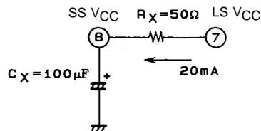
This measure yields an SVRR of approximately 50 dB. Note that the Rx loss voltage is approximately 1 V, and the  $P_O$  loss is about 1.0 to 1.5 W (to the 15 W level).
