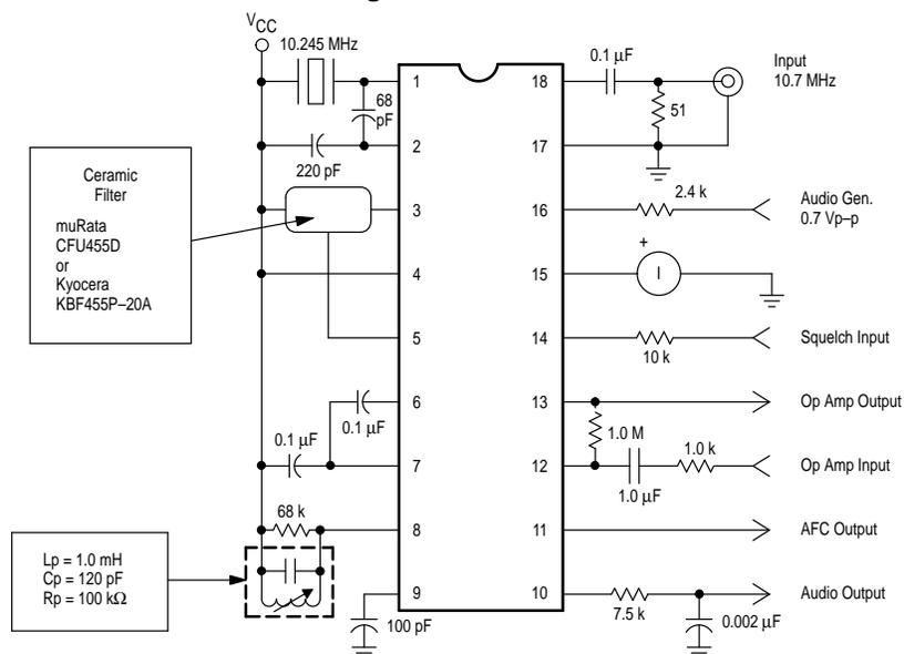
Figure 4. Mixer Voltage Gain
