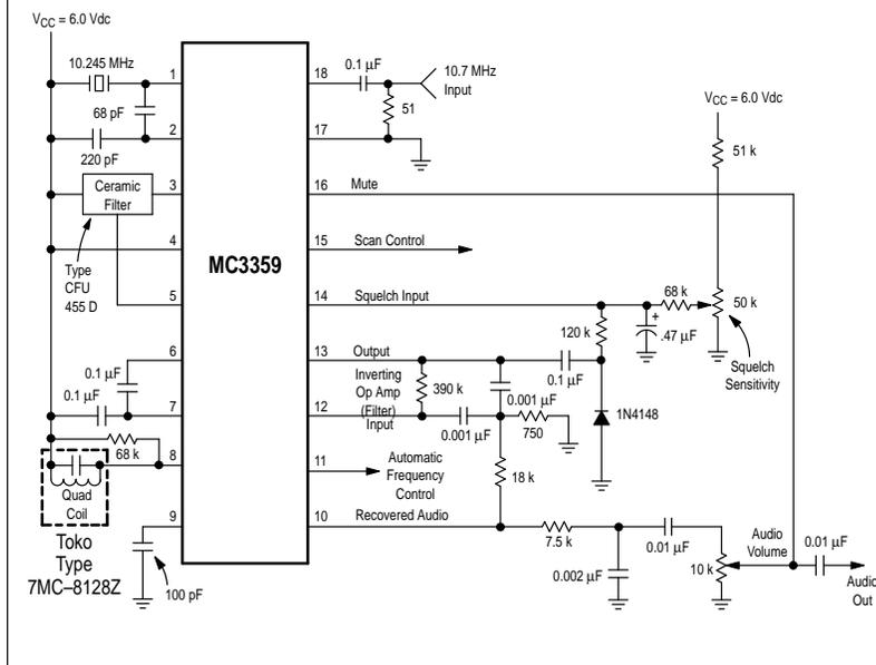
**Figure 2. Pin Connections and Functional Block Diagram**
