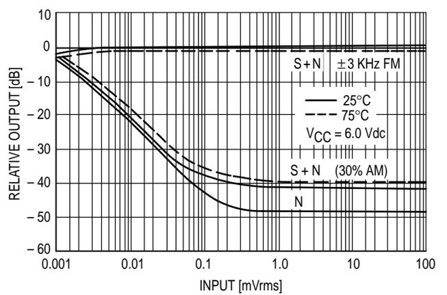
Figure 10. Output Components of Signal, Noise, and Distortion
