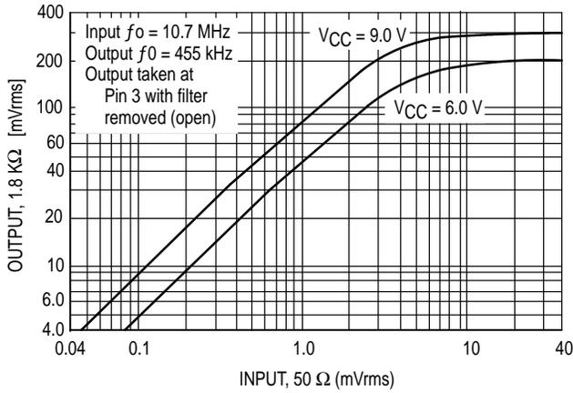
Figure 5. Limiting IF Frequency Response
