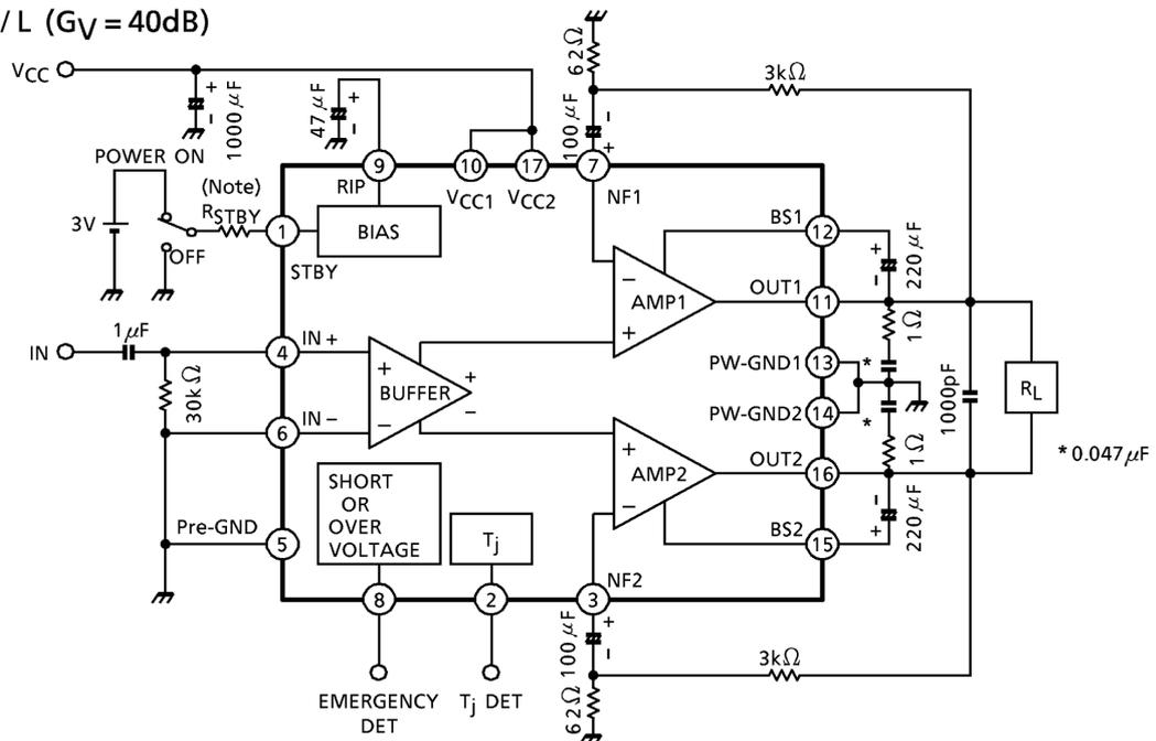
(Note) The purpose of  $R_{STBY}$  is current limiting resistance.
