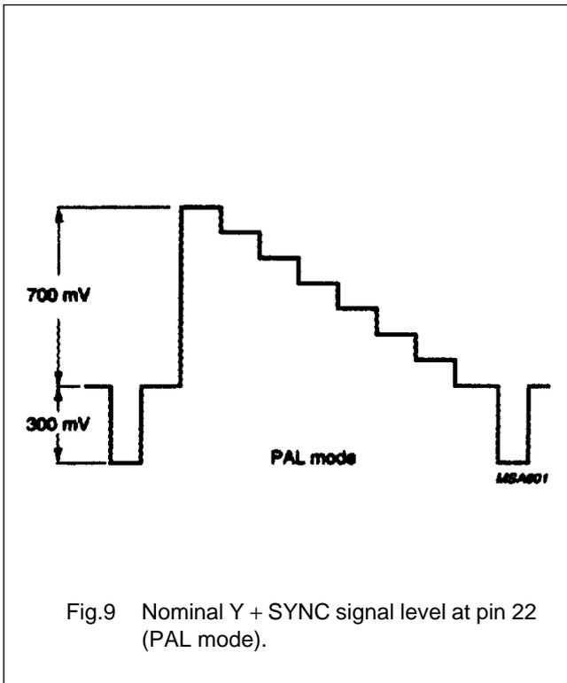
Fig.9 Nominal Y + SYNC signal level at pin 22 (PAL mode).
