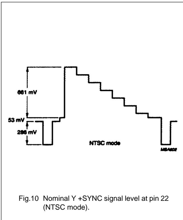
Fig.10 Nominal Y + SYNC signal level at pin 22 (NTSC mode).
