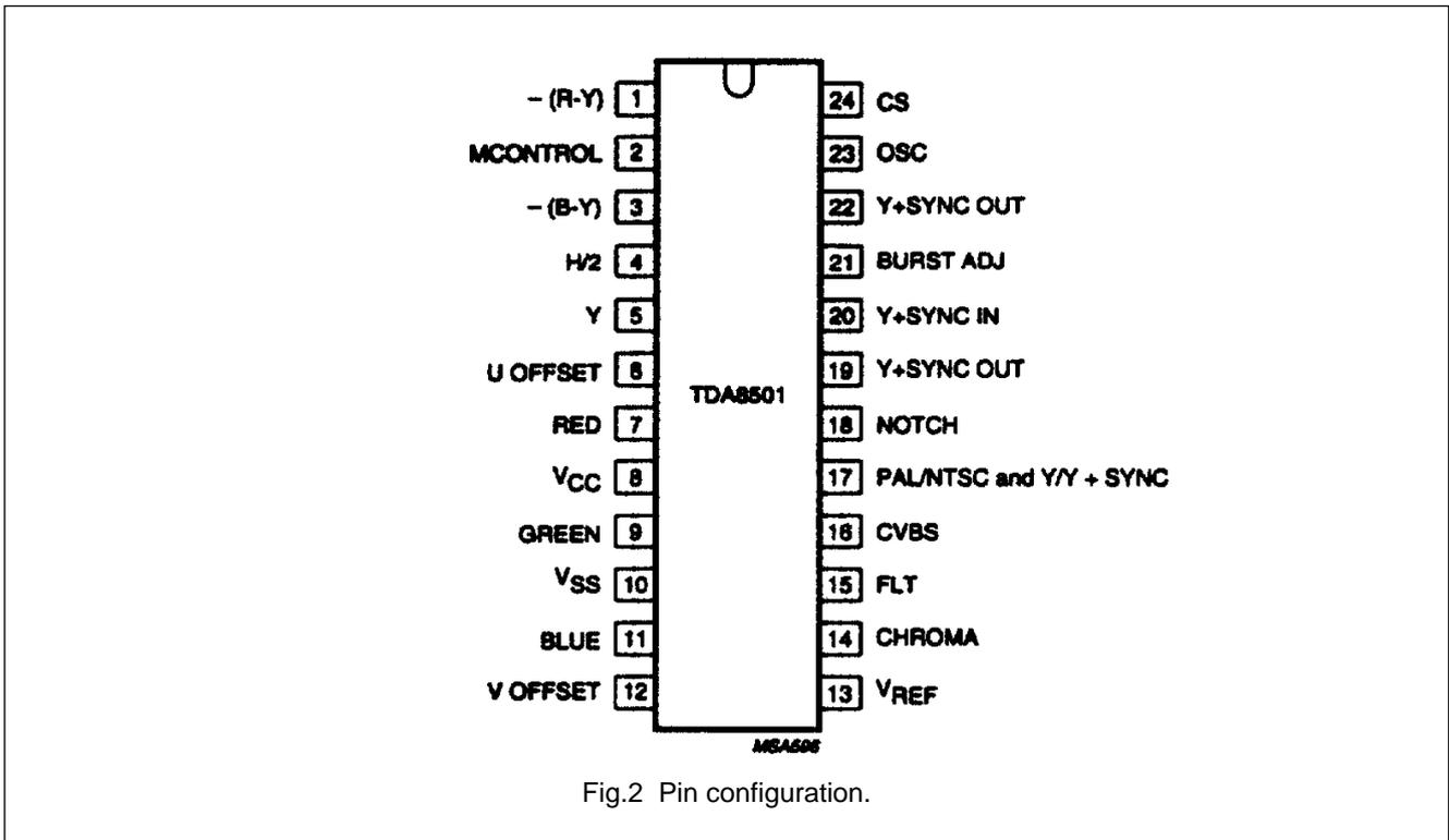
Fig.2 Pin configuration.
