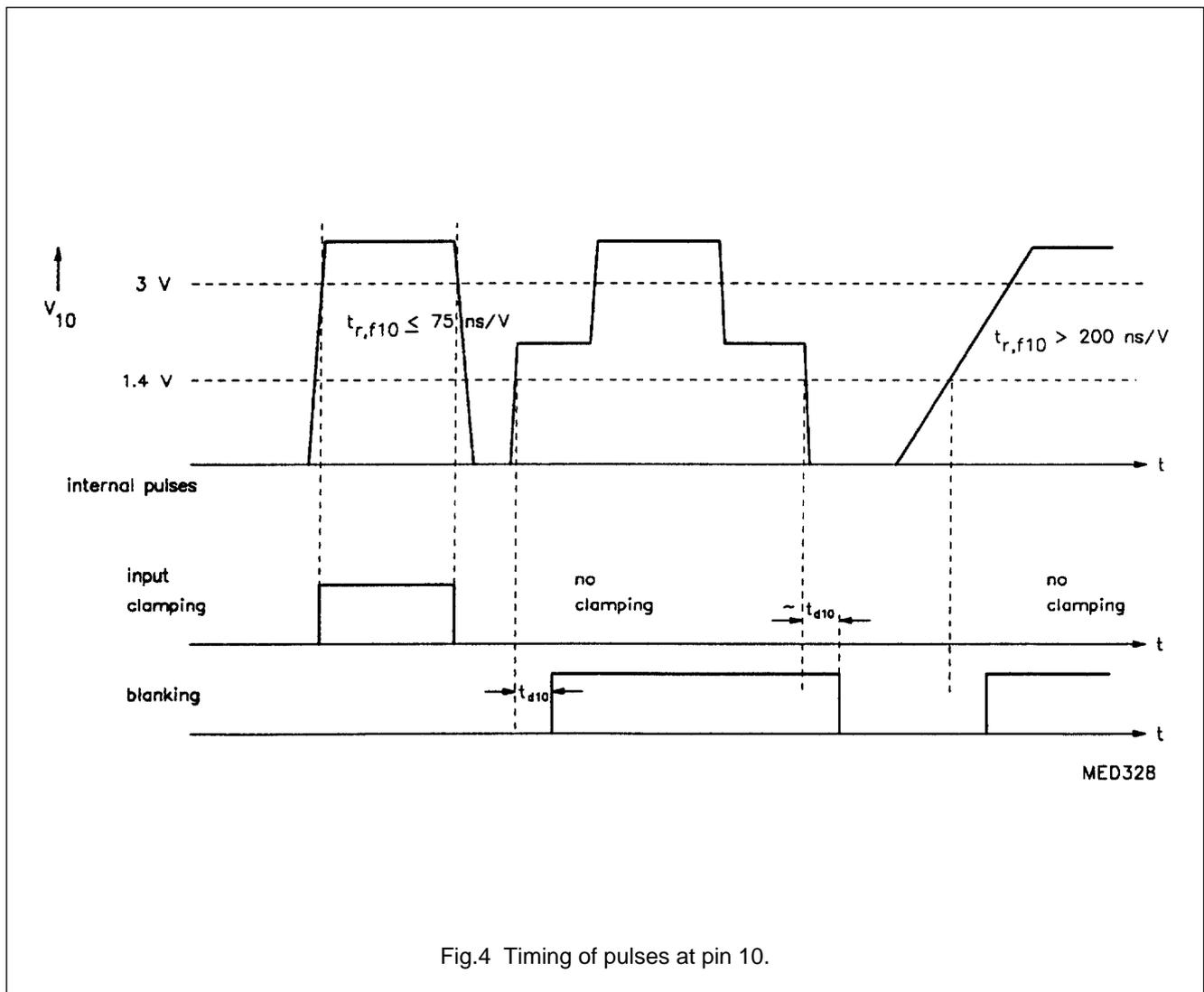
Fig.4 Timing of pulses at pin 10.
