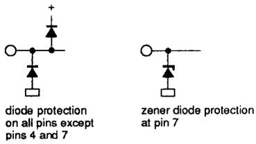
Fig.3 Internal circuits.
