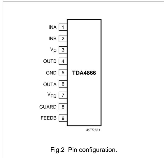
Fig.2 Pin configuration.
