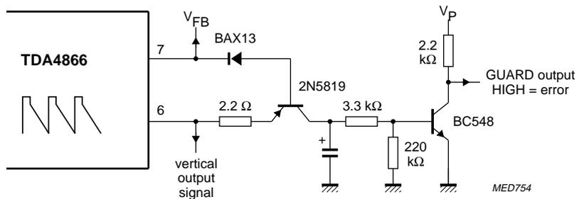
Fig.6 Application circuit for external guard signal generation.
