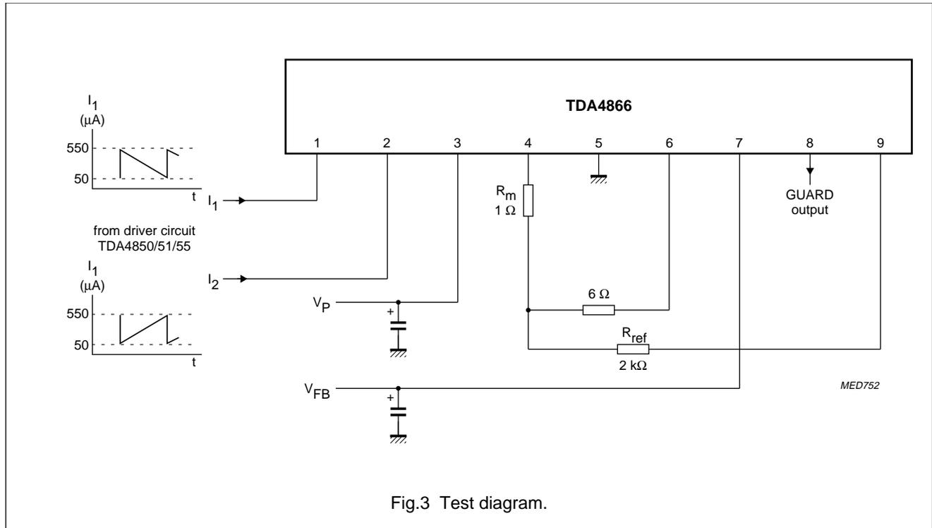
Fig.3 Test diagram.
