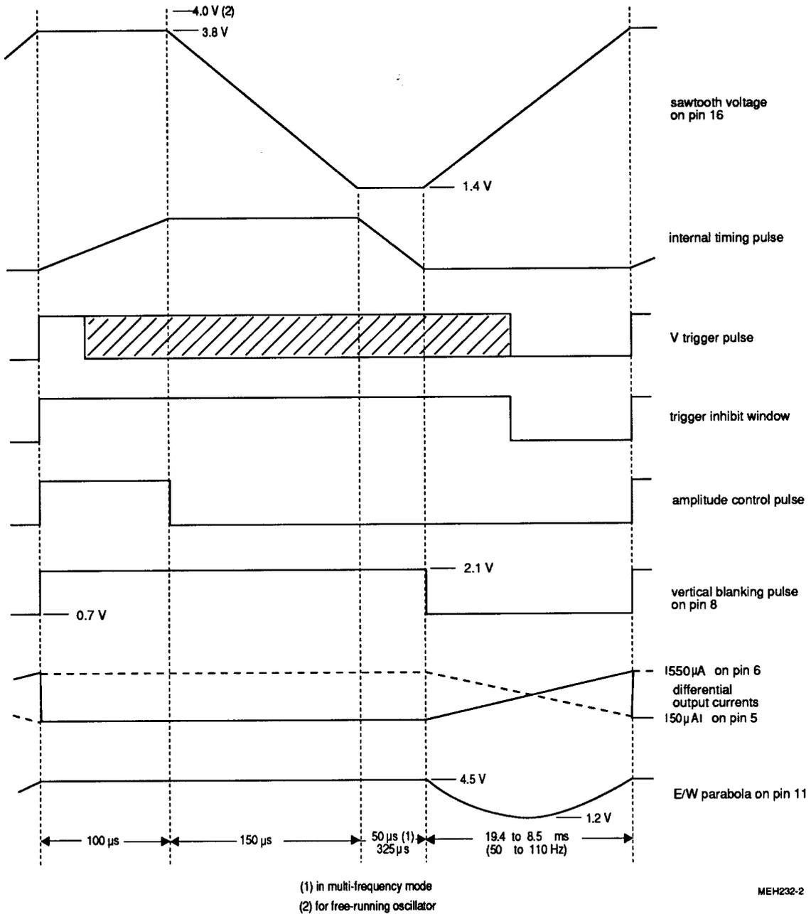
Fig.5 Vertical and E/W timing diagram.
