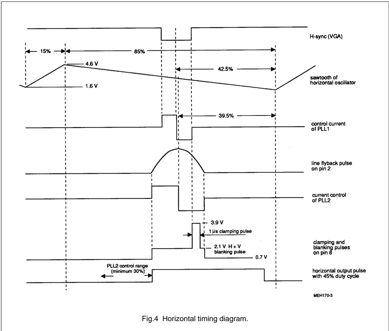
Fig.4 Horizontal timing diagram.
