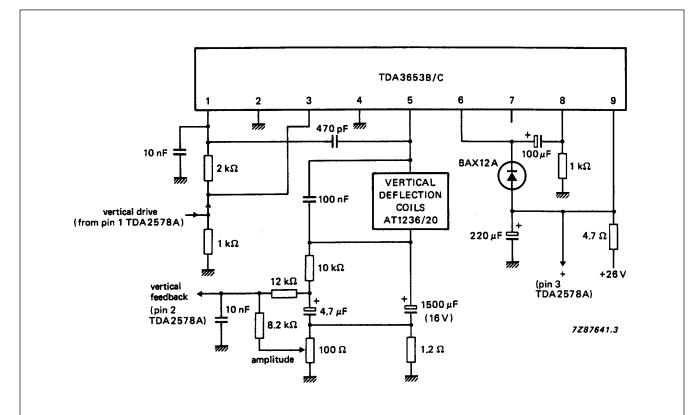
Note to deflection coils AT1236/20: L = 29 mH, R = 13.6  $\Omega$ ; deflection current without overscan is 0.82 A peak-to-peak and EHT voltage is 25 kV.
