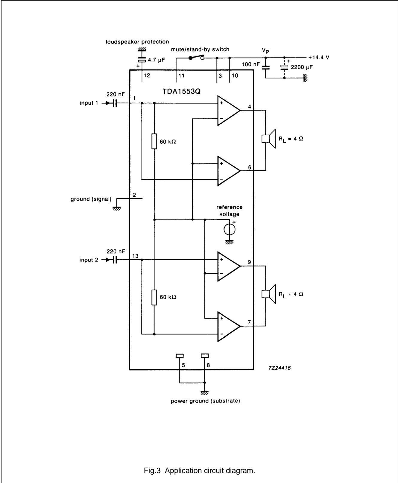
Fig.3 Application circuit diagram.
