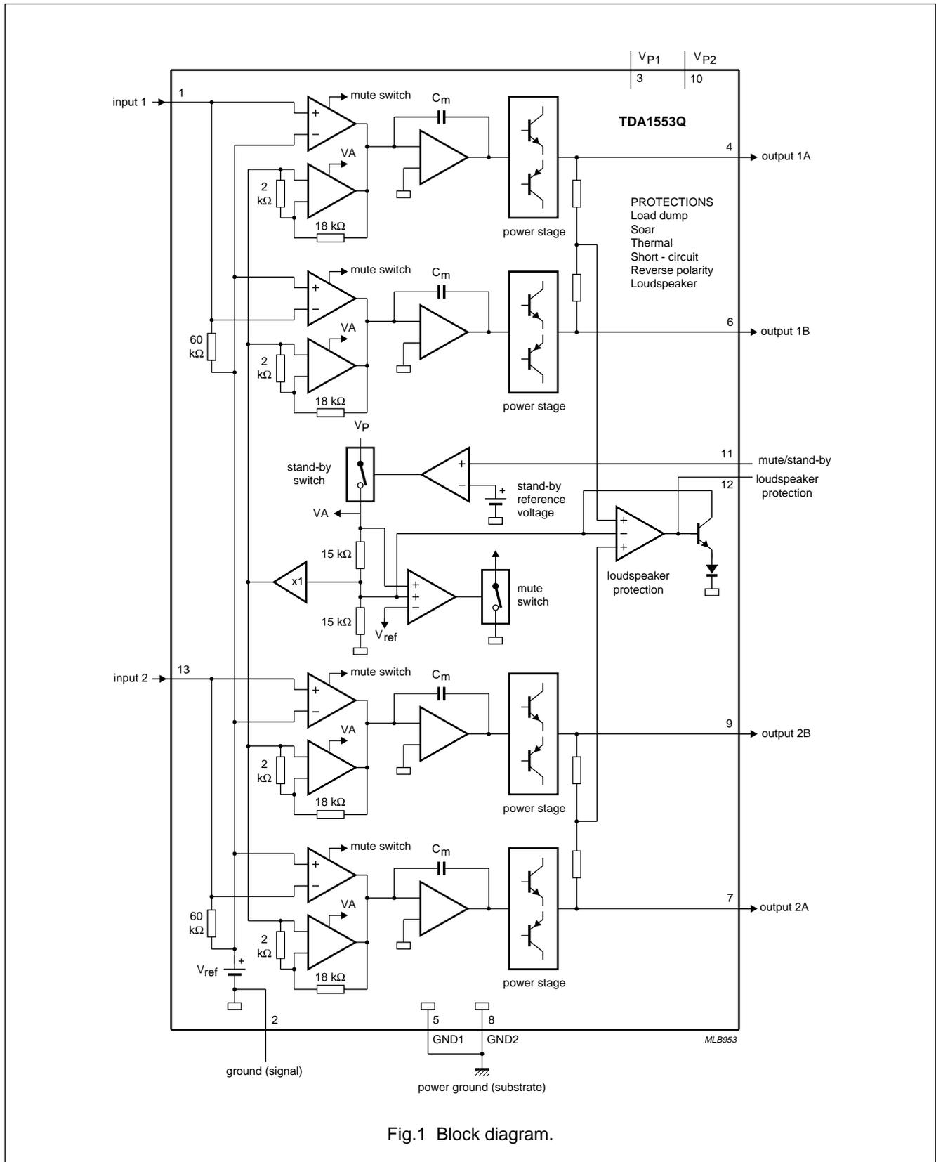
Fig.1 Block diagram.
