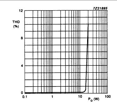
Fig.7 Total harmonic distortion (THD) as a function of output power ( $P_0$ ) for BTL application at  $R_L = 4 \Omega$ ; f = 1 kHz.
