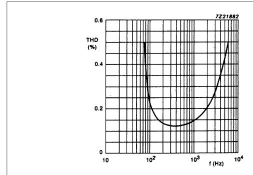
Fig.8 Total harmonic distortion (THD) as a function of operating frequency (f) for BTL application at  $R_L = 4 \Omega$ ;  $P_o = 1 \text{ W}$ .
