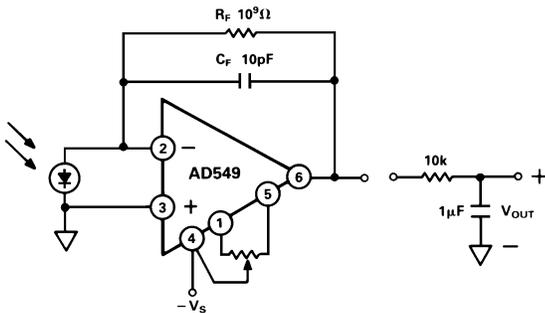
Figure 41. Photodiode Preamp
