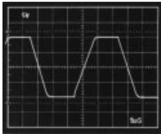
Figure 22. Unity Gain Inverter Large Signal Pulse Response
