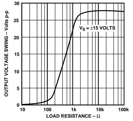
Figure 3. Output Voltage Swing vs. Load Resistance
