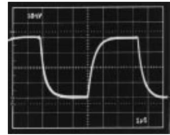
Figure 23. Unity Gain Inverter Small Signal Pulse Response
