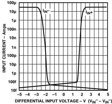
Figure 36. Input Current vs. Differential Input Voltage
