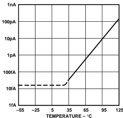
Figure 24. AD549 Input Bias Current vs. Ambient Temperature
