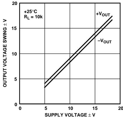
Figure 2. Output Voltage Swing vs. Supply Voltage
