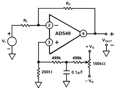
Figure 31. Alternate Offset Null Circuit for Inverter
