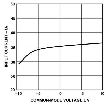
Figure 9. Input Bias Current vs. Common-Mode Voltage
