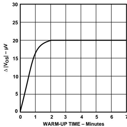
Figure 8. Change in Offset Voltage vs. Warm-Up Time
