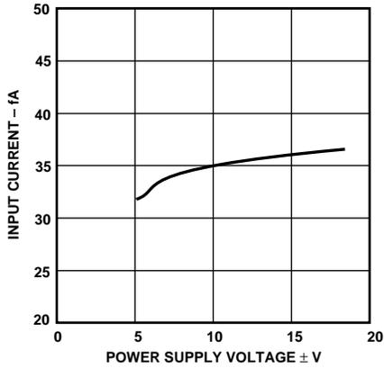
Figure 10. Input Bias Current vs. Supply Voltage
