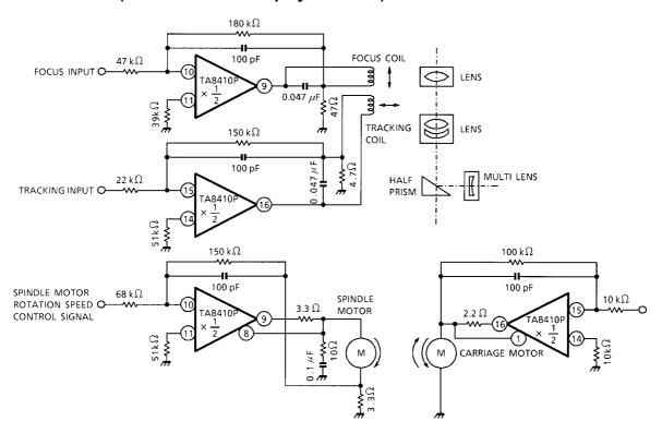
Note: Utmost care is necessary in the design of the output line, V<sub>CC</sub> and V<sub>EE</sub> line since IC may be destroyed due to short–circuit between outputs, air contamination fault, or fault by improper grounding.
