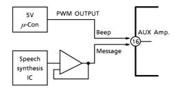
(Fig.7) The application of AUX. amplifier
