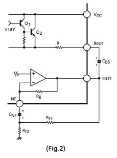
(1) In-phase and negative phase NF capacitor charging time
