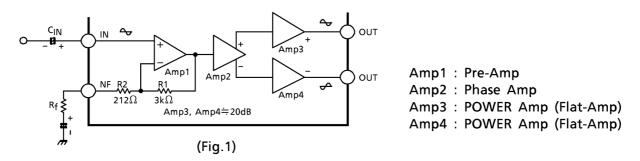
This IC has the amplifier constructions as shown Fig.1. The pre-amp (amp1) is provided to the primary stage, and the input voltage is amplified by the flat amps, amp3 and amp4 of each channel through the phase amp (amp2).
