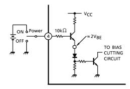
(Fig.3)With 4 pin set to high, power is turned ON.
