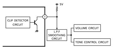
(Fig.5) ①pin: Open collector output (Active low)
