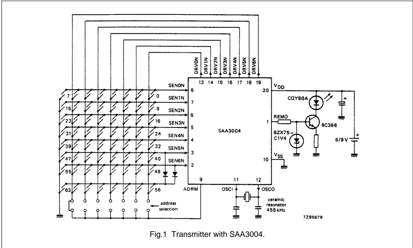
Fig.1 Transmitter with SAA3004.
