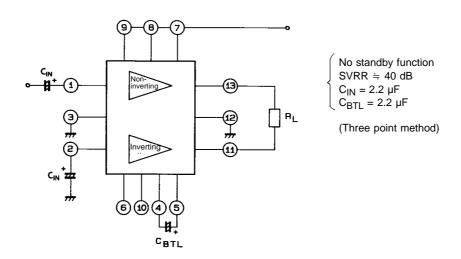
Dual-mode short-circuit test circuit
