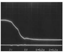
$V_{CC}=13.2$  V, standby supply +5 V,  $R_L=4~\Omega,~Rg=0$  Main switch ON/OFF test
