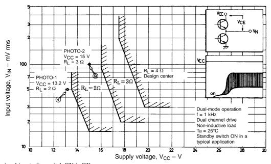
Strong signal input after switch-ON is OK. In BTL-mode operation, the load is  $R_{\rm L} \times 2$
