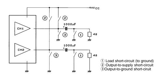
• Taking BTL coupling into consideration, the output-to-supply/output-to-ground protector is two-sided in order to protect both the IC and the speaker.
