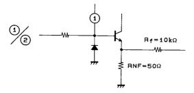
• Output pin 11/13 IC internal circuit
