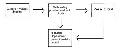
When using this method (simultaneously shorting the outputs to supply and to ground) In BTL mode, the IC protection function works even in noninverted output  $\rightarrow$  output-to-supply mode, inverted output  $\rightarrow$  output-to-ground mode. (The reverse is also OK.)
