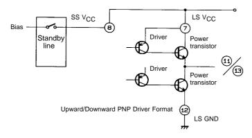
• The minimum configuration for dual-mode operation
