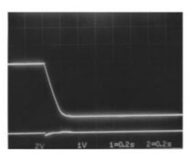
$V_{CC}=13.2$  V, standby supply +5 V,  $R_L=4~\Omega,~Rg=0$  Standby switch ON/OFF text
