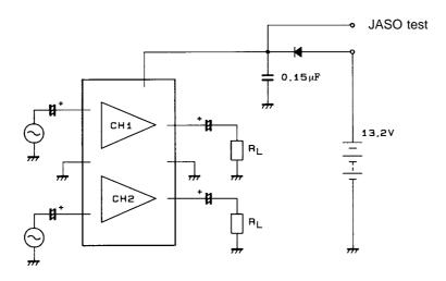
The power supply line positive surge breakdown margin has been increased by using the built-in overvoltage protection circuits  $(V_{CCX} = 28 \text{ V})$  to cut off all bias circuits/change the base-emitter reverse of the output stage. In other words, the breakdown margin is being raised by changing output stage groups that operate as the  $V_{CEO}$  ( $V_{CER}$ ) type to the  $V_{CES}$  ( $V_{CBO}$ ) type.
