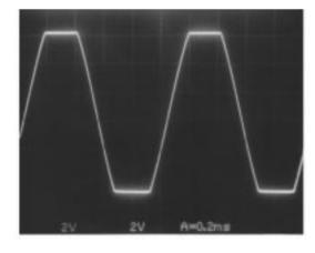
$$\begin{split} &V_{CC}=13.2 \text{ V}, \\ &R_L=4 \ \Omega, \\ &Rg=600 \ \Omega, \\ &THD=10\%, \\ &f=1 \text{ kHz}, \\ &Output \ DC \ waveform \end{split}$$
